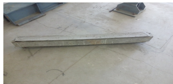
Fig. 3: After bonding of beam specimen and ferrocement plate
